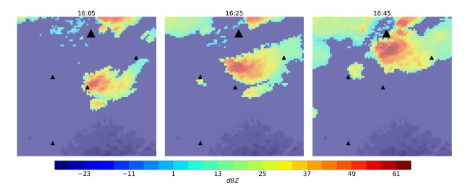
Fig. 10 Images depict Z near the city of Pavia at 16:05 (left), 16:25 (centre), and 16:45 (right). Each image covers a surface of  $40 \times 40$  km<sup>2</sup> wherein Pavia is the centre (the central triangle) and the city of Milan is on top. Smaller triangles at the west, south-west, and north-east of Pavia represent the cities of Voghera, Tortona, and Lodi, respectively. The storm is quite isolated and moving northward. The greatest value of 64.5 dBZ is shown at 16:45
