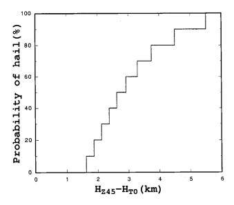
Fig. 3 Probability of hail (POH) as computed by Waldvogel. et al. (1979). POH is expressed as a function of the height difference between the echotop-45 (H<sub>45</sub>) and the melting level (H<sub>T0</sub>). This plot is obtained by Holleman (2001)
